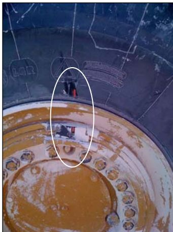
Red chalk mark which registers the rim and tire assembly
