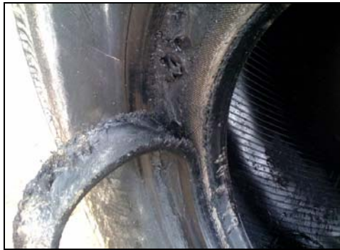
Bead damage due to bead and rim slip on 3 piece wheel assemblies
